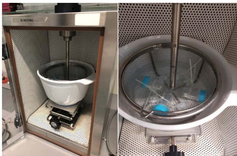
Appendix Fig. 1. Ultrasonic probe and samples set up.
