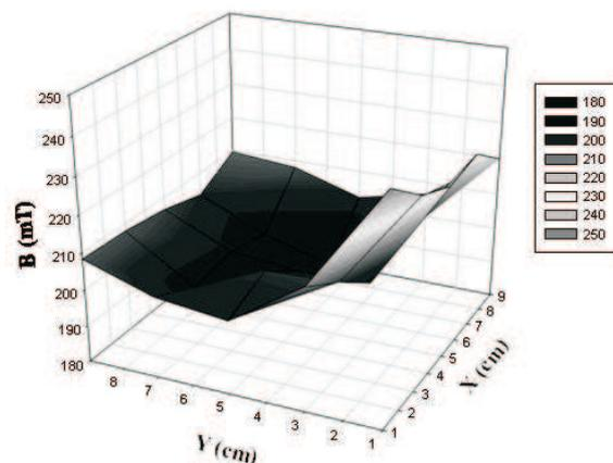
**Fig. 1.** Distribution of magnetic field between pole pieces of the electromagnet taken at 220 V.
