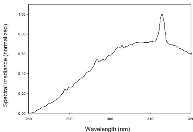
**Fig. 1.** Emission spectrum of the applied source of UV-B radiation, VL-115 M (Vilber Lourmat, France), normalized to maximum at 313 nm.
