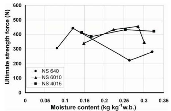
Fig. 6. Ultimate strength force versus seed moisture content during compressive testing of NS hybrids.
