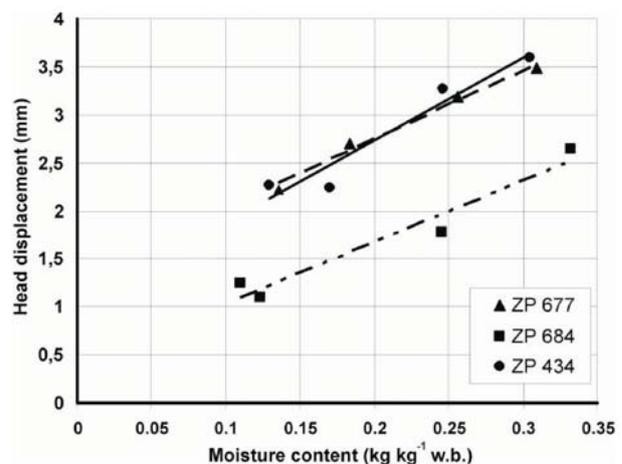
Fig. 7. Relationship between head displacement and moisture content for ZP hybrids (ZP 684:  $\delta_H=6.3979$ ,  $MC+0.3944$ ,  $R^2=0.944$ ; ZP 677:  $\delta_H=8.5447$ ,  $MC+1.0242$ ,  $R^2=0.9334$ ; ZP 434:  $\delta_H=7.1091$ ,  $MC+1.3264$ ,  $R^2=0.9864$ ).
