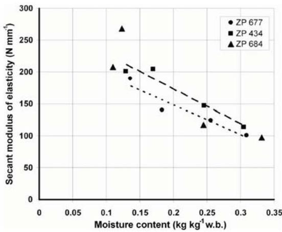
Fig. 9. Secant modulus of elasticity of ZP hybrids (ZP 434:  $E_s = -540.63 MC + 281.41$ ,  $R^2 = 0.940$ ; ZP 684:  $E_s = -686.47 MC + 311.48$ ,  $R^2 = 0.824$ ; ZP 677:  $E_s = -466.33 MC + 241.78$ ,  $R^2 = 0.911$ ).
