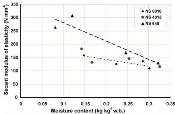
Fig. 10. Secant modulus of elasticity of NS hybrids (NS 640:  $E_s = -688.87 MC + 349.96$ ,  $R^2 = 0.867$ ; NS 4015:  $E_s = -252.31 MC + 199.89$ ,  $R^2 = 0.545$ ; NS 6010:  $E_s = -246.17 MC + 191.89$ ,  $R^2 = 0.677$ ).
