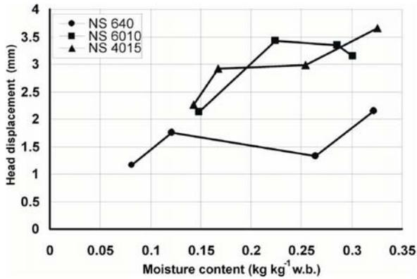
Fig. 8. Relationship between head displacement and moisture con-
