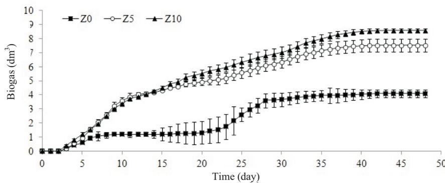
Fig. 1. Accumulated biogas production in all the treatments. The bars designate the values of the two replicates of each treatment.
