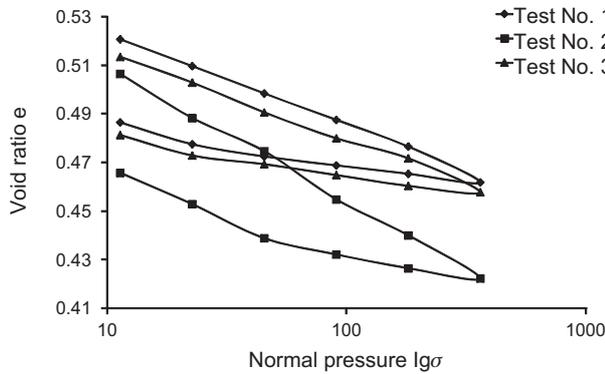
Fig. 4. Oedometer curves obtained for lentil vetch.
