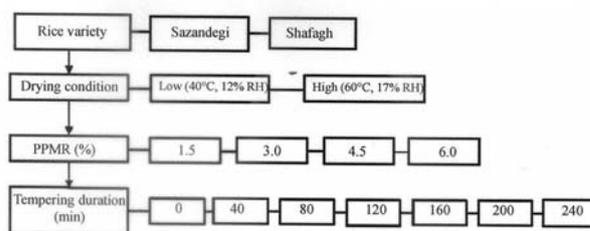
Fig. 1. Experimental design for drying and tempering operations.
