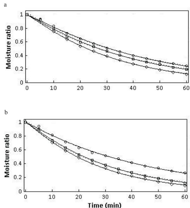
Fig. 2. Variation of the experimental and predicted moisture ratios by the Page model and Two-term model with baking time in: a – natural, b – forced convection modes (the Two-term model (---), the Page model (—)). Explanations as in Fig. 1.
