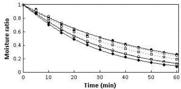
Fig. 1. Variation of the experimental and predicted moisture ratios by the Page model with baking time in both natural and forced convection mode (under natural convection (---):  $\circ$  180,  $\square$  200,  $\diamond$  220°C and under forced convection (—):  $\bullet$  180,  $\blacksquare$  200,  $\blacklozenge$  220°C.
