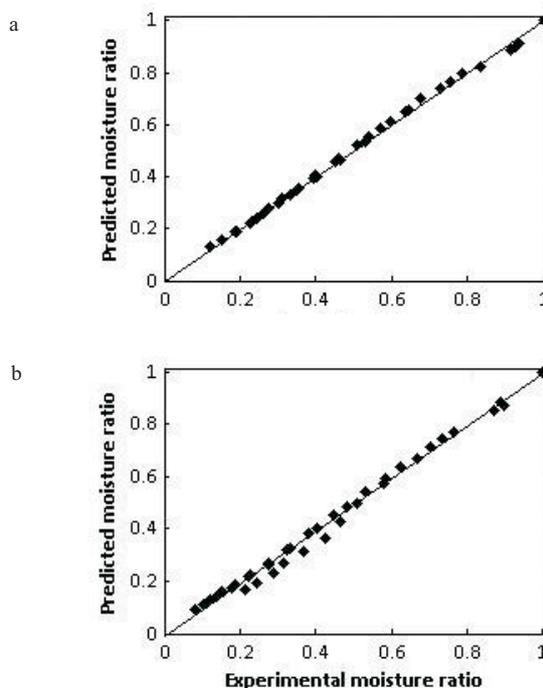
**Fig. 3.** Experimental and predicted moisture ratio in: a – natural and b – forced convection modes at all baking temperatures.
