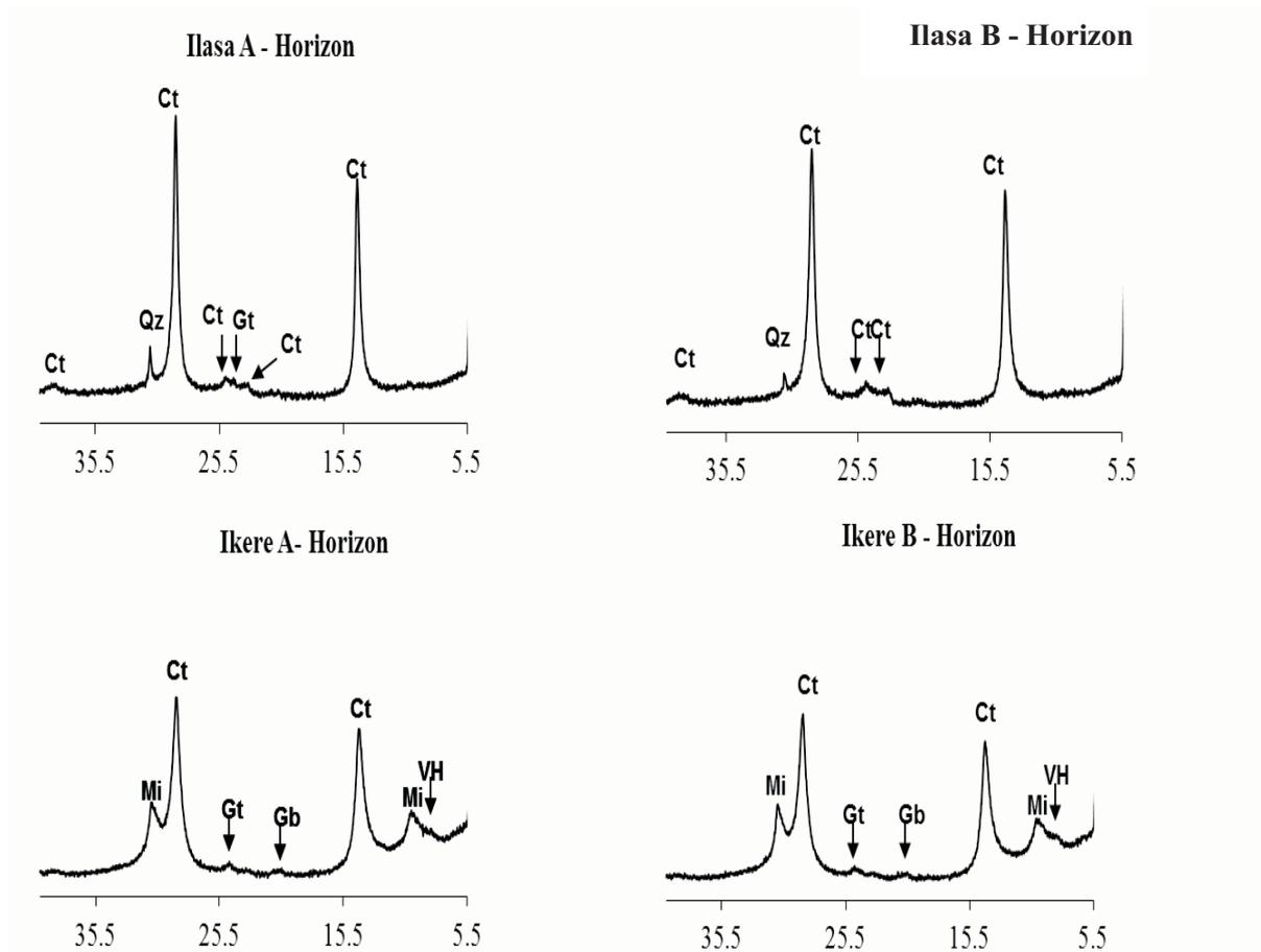
**Fig. 2.** Fine clay fraction X-ray diffractograms of the studied soils highlighting the mineral content and distribution. VH - hydroxy-interlayered vermiculite, Mi – mica, Ct – kaolinite, Gb – gibbsite, Gt – goethite, Qz – quartz.
