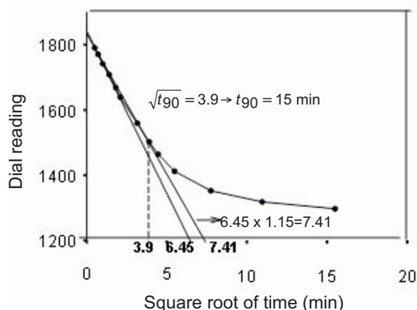
Fig. 1. Square root of time versus dial reading for establishing a 90% consolidation point.
