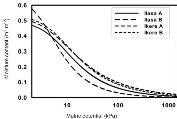
**Fig. 3.** Moisture retention by clay fraction samples from the various sites.
