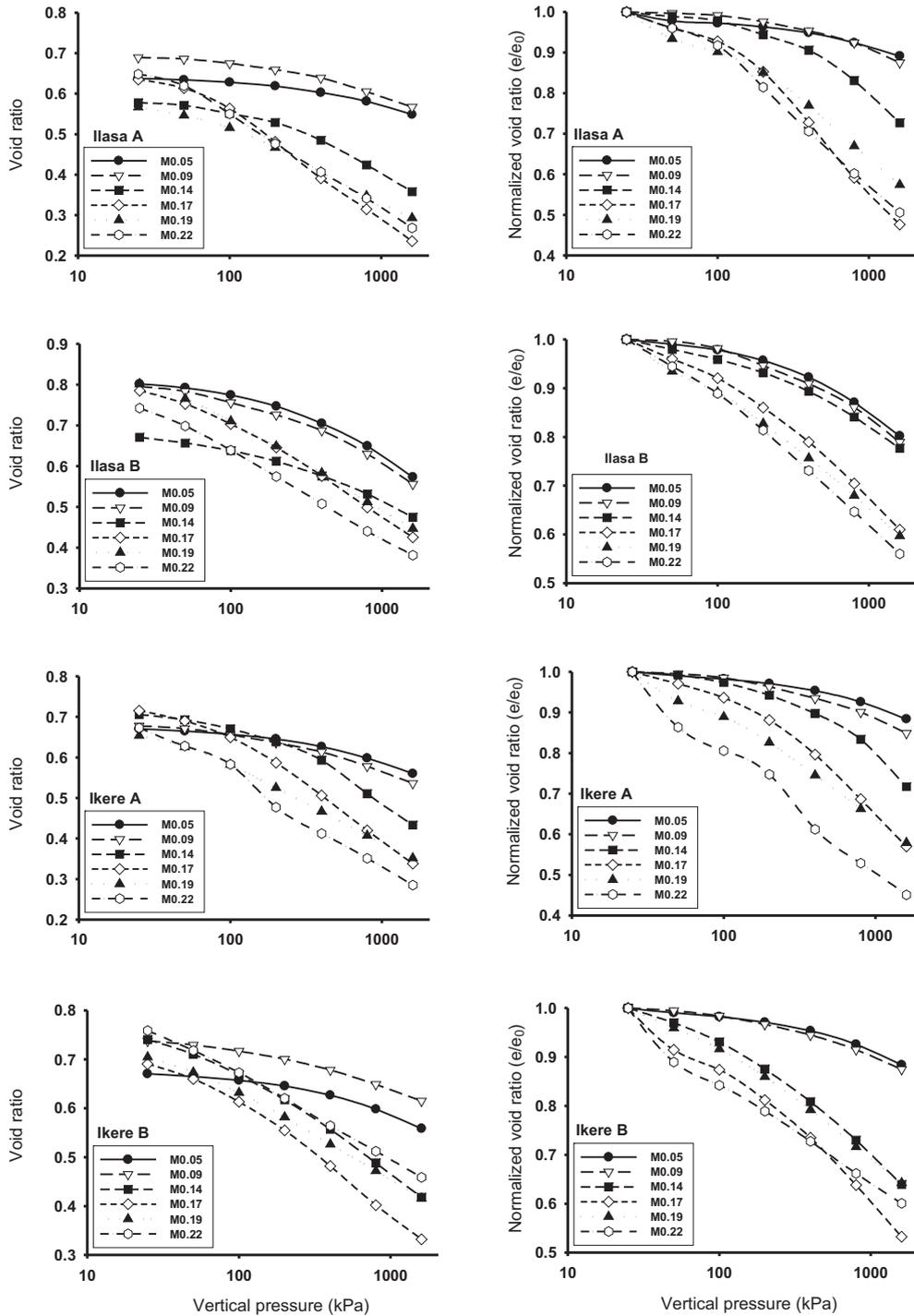
Fig. 4. Stress vs. void ratio responses for the studied samples at 6 uniform moisture contents.
