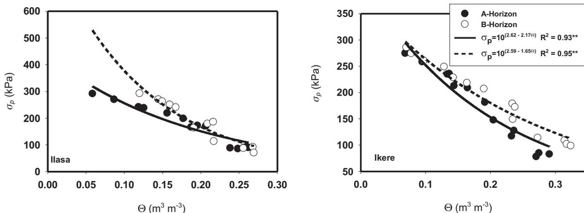
Fig. 5. Load bearing capacity curves of the studied soils.
