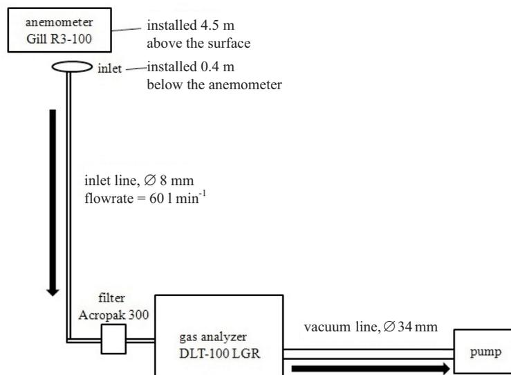
**Fig. 2.** Scheme of the eddy covariance system for measuring methane. The arrows indicate the direction of the intake air.
