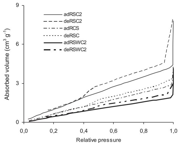
Fig. 2. Hysteresis loop for rapeseed oil cake and its mixtures with wheat meal. Abbreviations: see in the text.
