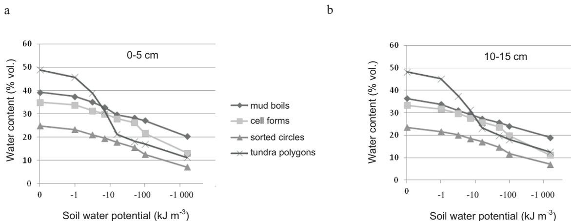
**Fig. 2.** Relationship between soil water potential and water content (% vol.) at: a – 0-5 and b – 10-15 cm for soils formed on different micro-relief forms.
