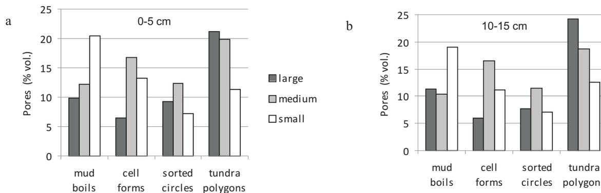
**Fig. 3.** Content of pores (% vol.) of different size at: a – 0-5 and b – 10-15 cm in the investigated micro-relief forms; large pores – dia > 50  $\mu\text{m}$ , medium pores – 50  $\mu\text{m}$  > dia > 0.2  $\mu\text{m}$ , small pores – dia < 0.2  $\mu\text{m}$ .
