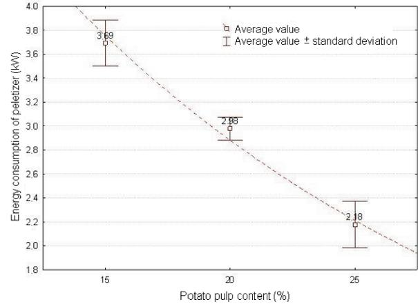
Fig. 1. The influence of potato pulp content in a mixture with oat bran on the power demand of the pellet mill.
