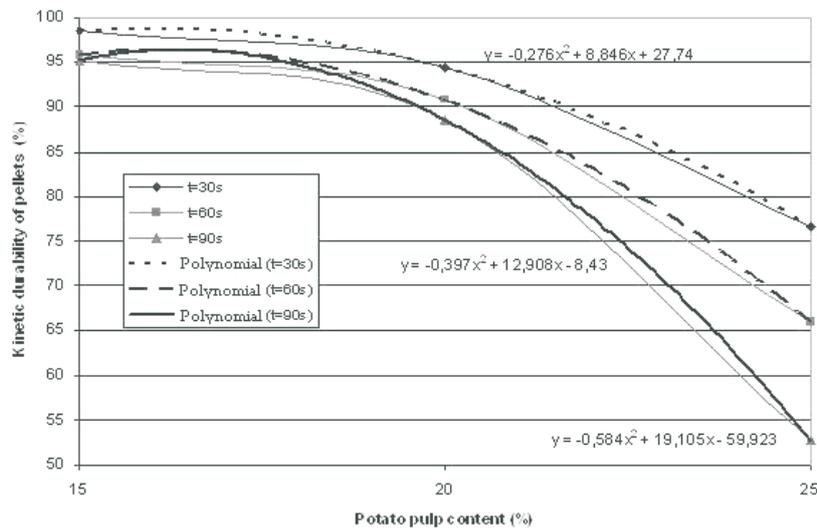
**Fig. 3.** The influence of potato pulp content in a mixture with oat bran on the kinetic durability of the pellets determined using Holmen method.
