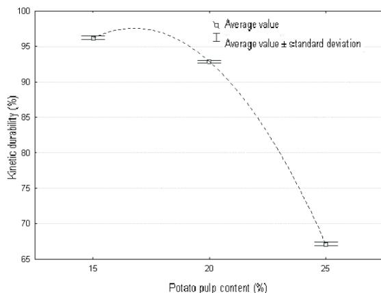
**Fig. 4.** The influence of potato pulp content in a mixture with oat bran on the kinetic durability of the pellets determined using Pfof method.
