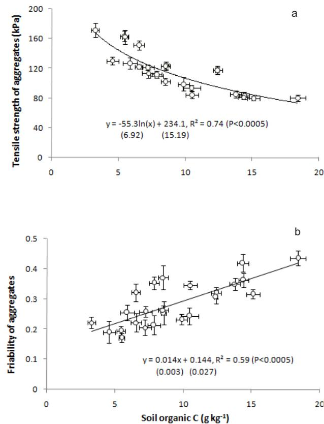
**Fig. 2.** Relations between: a – tensile strength and b – friability of aggregates and soil organic carbon (SEE at 5% associated with the coefficients are given in parentheses). SEE stands for standard error of estimates. It is a measure of prediction accuracy and is calculated as the difference between actual and predicted values.
