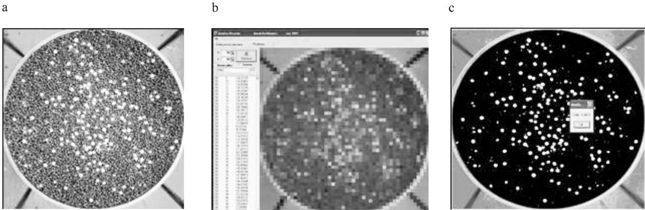
**Fig. 1.** Image of a selected cross-section of the analytical silo in the subsequent stages of computer image analysis: a – digital image, b – image after pixelisation of cells 50x50, c – binary image.
