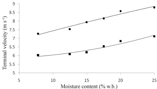
**Fig. 1.** Terminal velocity variation versus seed moisture content: ● grade A, ■ grade B.
