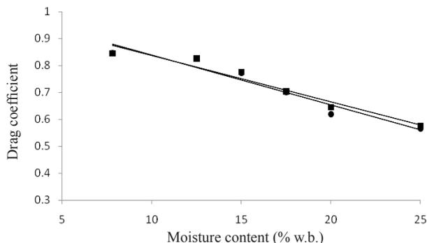
**Fig. 2.** Drag coefficient variation versus seed moisture content. Explanation as in Fig. 1.
