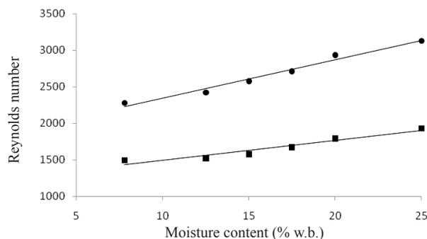
**Fig. 3.** Reynolds number variation versus seed moisture content. Explanation as in Fig. 1.
