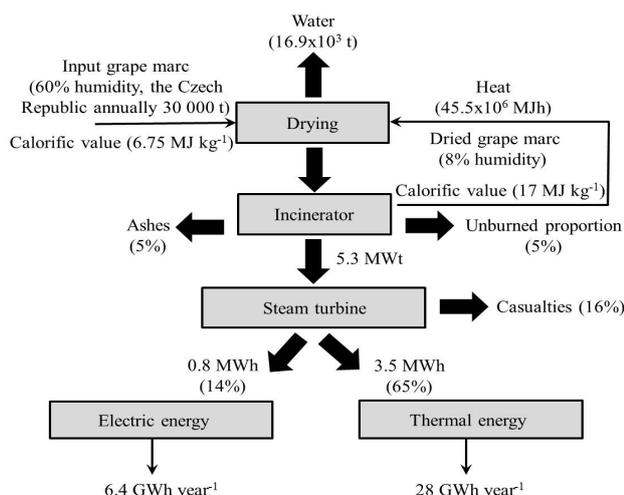
Fig. 3. Scheme of mass and energy balances for pomace in the Czech Republic.
