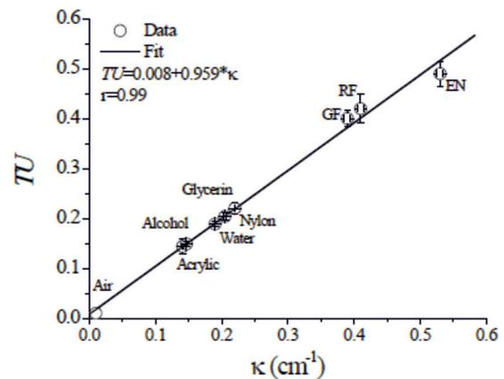
**Fig. 2.** CT calibration curve for  $^{241}\text{Am}$  gamma-ray radioactive source. Error bars represent the measurement standard deviation. The value 0.959 is the parameter  $\alpha$  (inclination of straight line) of Eq. (2), which relates the tomography unit ( $TU$ ) and the soil physical properties.
