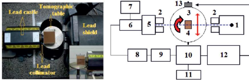
**Fig. 1.** Picture of the  $\gamma$ -ray CT scanner and its schematic diagram: 1 – radioactive source, 2 – lead collimator, 3 – tomographic table, 4 – soil sample, 5 – NaI(Tl) scintillation detector, 6 – photomultiplier tube, 7 – high voltage unit, 8 – amplifier, 9 – single channel analyzer, 10 – counter, 11 – timer, 12 – PC, 13 – stepper motor controls. Adapted from Pires *et al.* (2002, 2011a).
