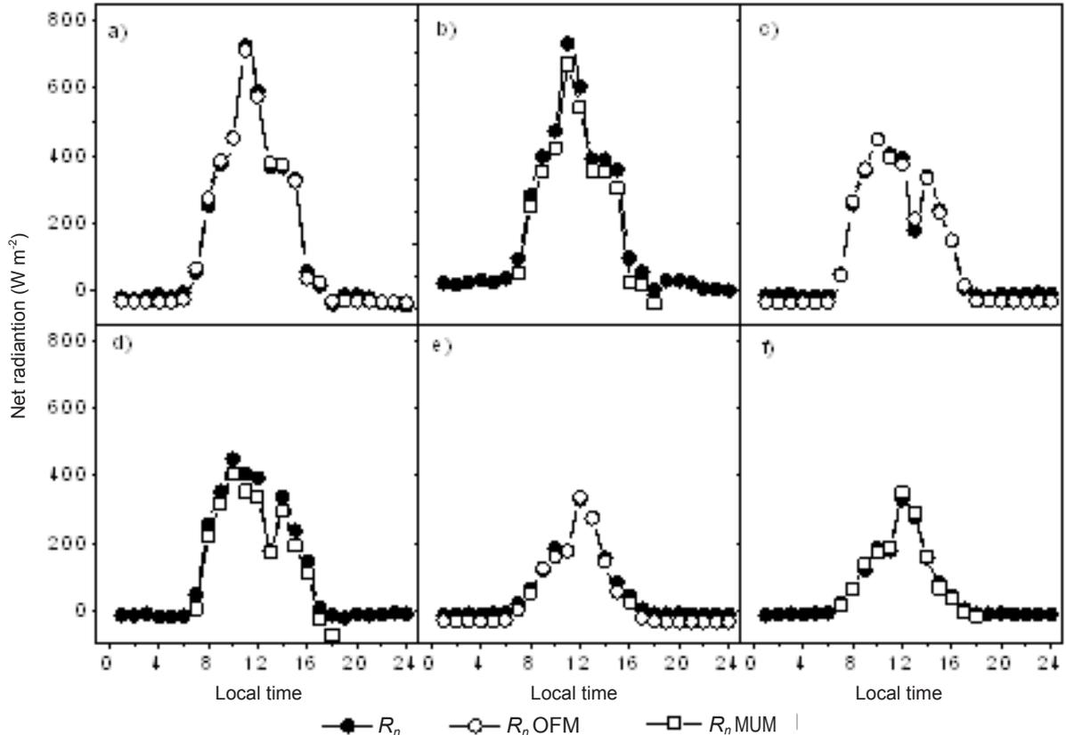
**Fig. 8.** Net radiation as observed ( $R_n$ ), and estimated by: the Ortega-Farias ( $R_n$  OFM) model, the Monteith and Unsworth ( $R_n$  MUM) under clear sky condition (a,b,c,d) and partially cloudy sky (e, f) during the mid-season stage.
