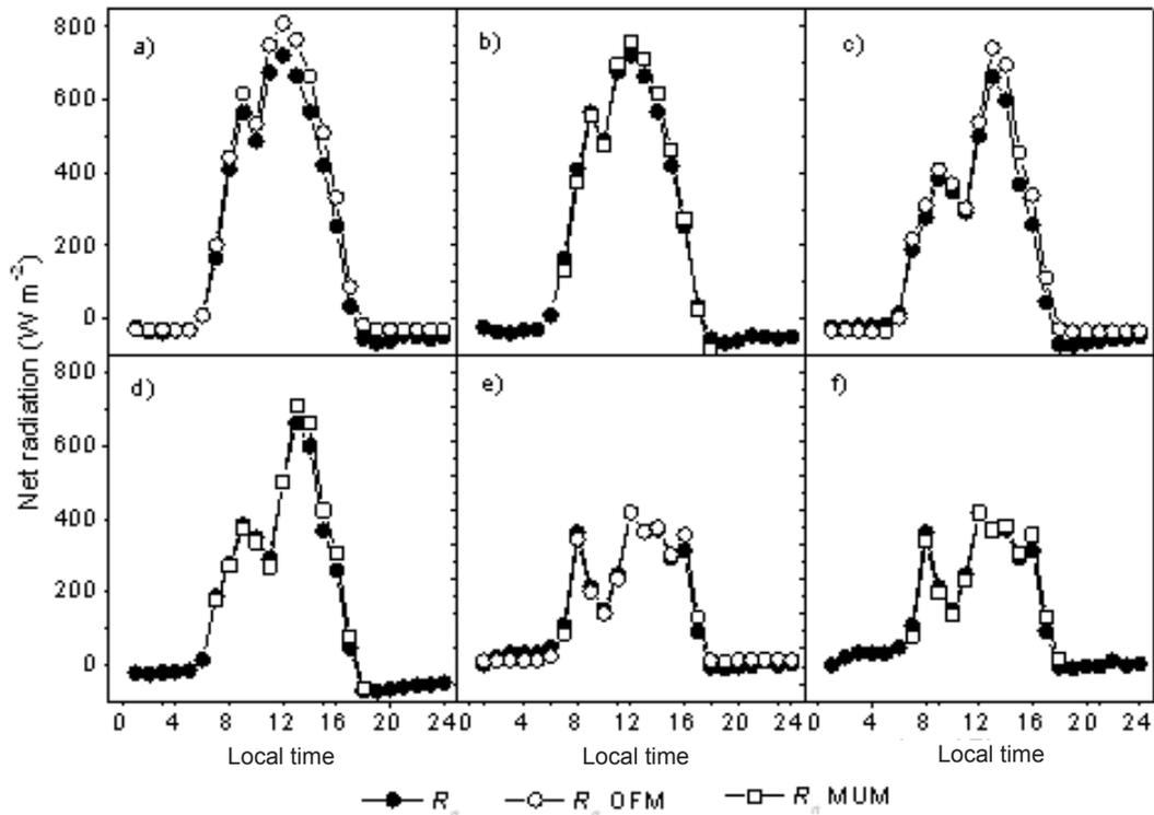
**Fig. 7.** Net radiation as observed ( $R_n$ ), and estimated by: the Ortega-Farias ( $R_n$  OFM) model, the Monteith and Unsworth ( $R_n$  MUM) under clear sky condition (a,b) and partially cloudy sky (c,d,e,f) during the crop development stage.
