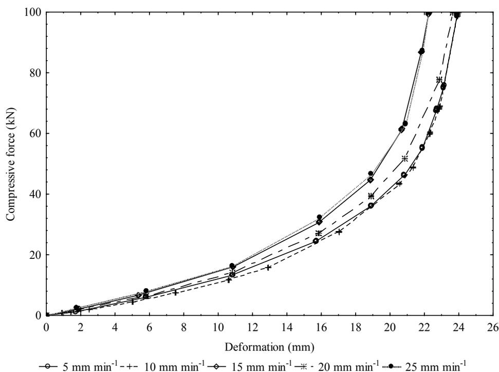
**Fig. 1.** Dependency between compressive force and deformation curves of bulk unroasted kernels in relation to different speed, similar to roasted bulk kernels.
