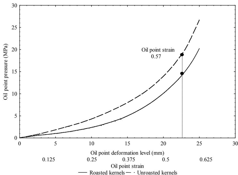
**Fig. 2.** Oil point pressure versus deformation level and strain of bulk roasted and unroasted kernels at pressing height 40 mm and speed  $5 \text{ mm min}^{-1}$ .
