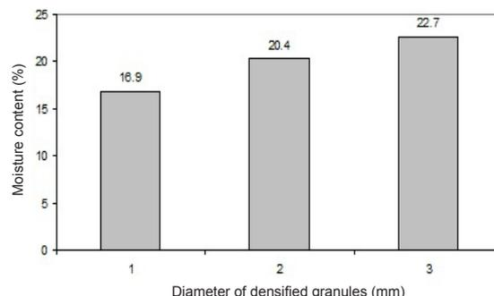
**Fig. 6.** Correlation between moisture content and the size of particles of pellets from a mixture of nettle waste and a 5% potato starch solution obtained in a non-pressure way.
