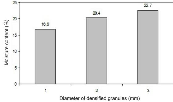
**Fig. 6.** Correlation between moisture content and the size of particles of pellets from a mixture of nettle waste and a 5% potato starch solution obtained in a non-pressure way.
