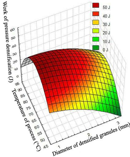
**Fig. 4.** Effect of material (the size of fraction particles) and process (the temperature of the process) factors on the work of open-chambered pressure densification of pellets (obtained in a non-pressure manner through enveloping) from a mixture of nettle waste and a 5% potato starch solution.
