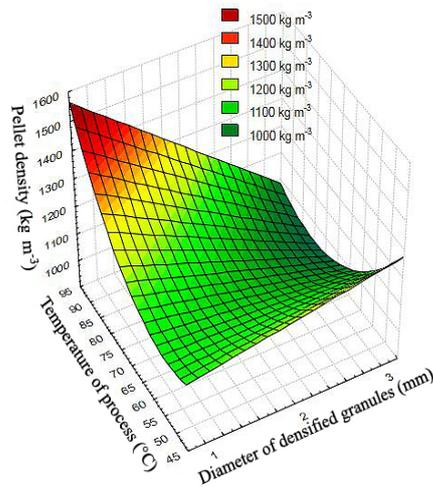
**Fig. 5.** Effect of material and process factors (the diameter of particles of the densified fraction and process temperature) on the density of pellets obtained in the process of open-chambered pressure agglomeration, of pellets (obtained in a non-pressure way) from nettle waste and a 5% potato starch solution.
