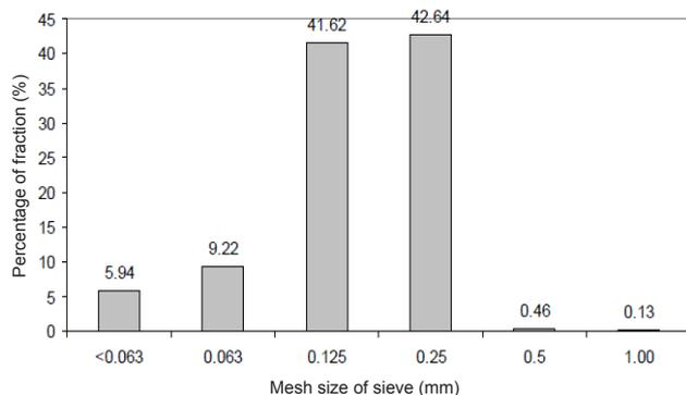
**Fig. 1.** Granulometric distribution of particles of shredded nettle waste subjected to a sieve analysis.
