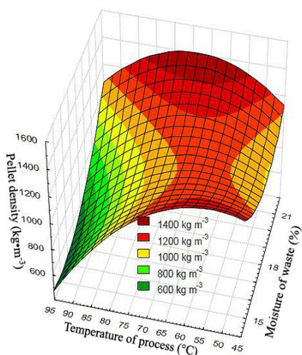
**Fig. 3.** Influence of material and process factors (the temperature of the process and the moisture content in pellets) on the density of pellets obtained in the process of open-chambered nettle waste pressure densification.
