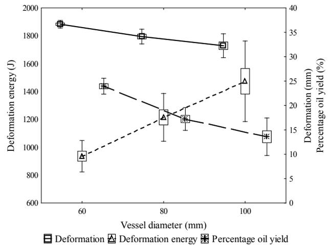
**Fig. 1.** Box plot of deformation, deformation energy and percentage oil yield versus vessel diameter.
