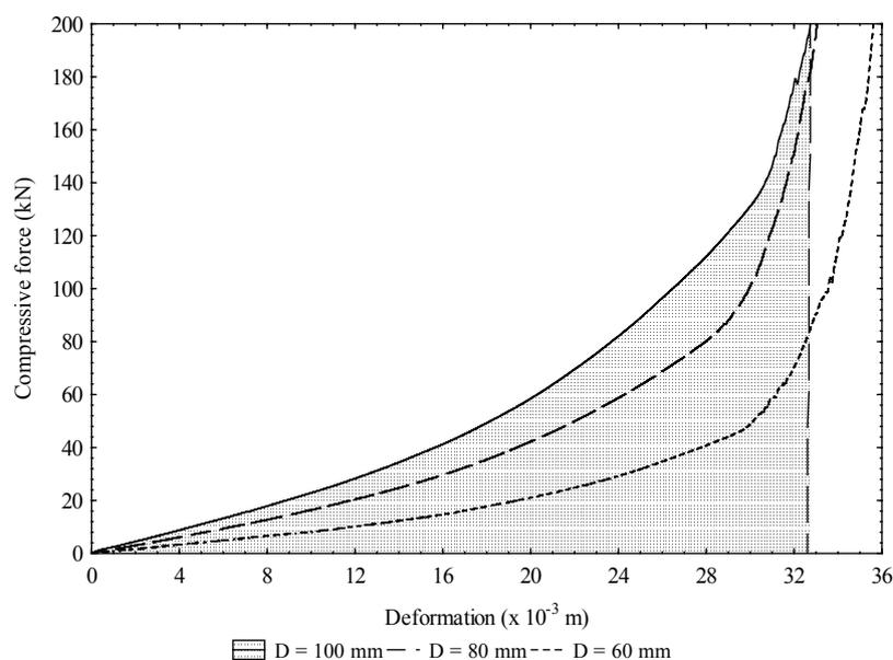
**Fig. 2.** Dependency between compressive force and deformation curves of non-roasted bulk oil palm kernels in relation to the vessel diameters ( $D$ ).
