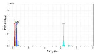
Fig. 1. EDX spectrum of the Fe-ALA nano-sized complex.
