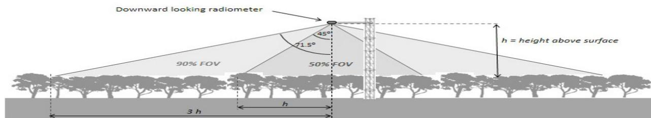
**Fig. 1.** Representation of limits of the areas corresponding to the field of view (FOV) contributing to 50 and 90% of total signal for a downward looking radiometer with 180° FOV and cosine response.
