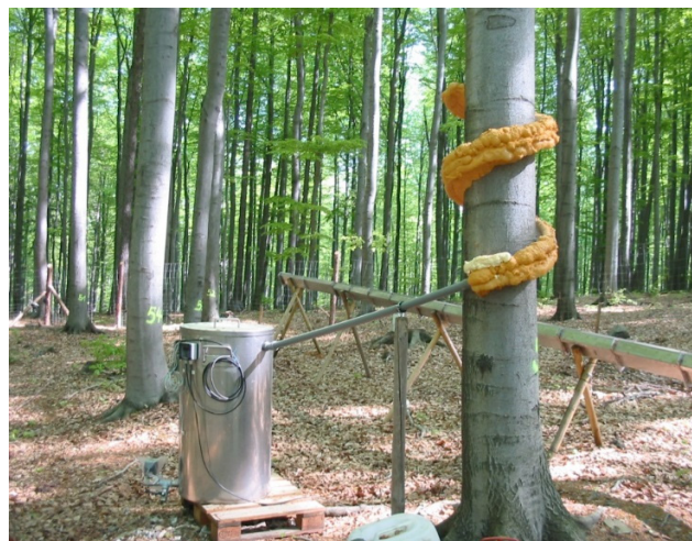
Fig. 2. Automated stemflow collector at the BULB (Beech Stand Landberg) beech site, TU Dresden, Germany.
