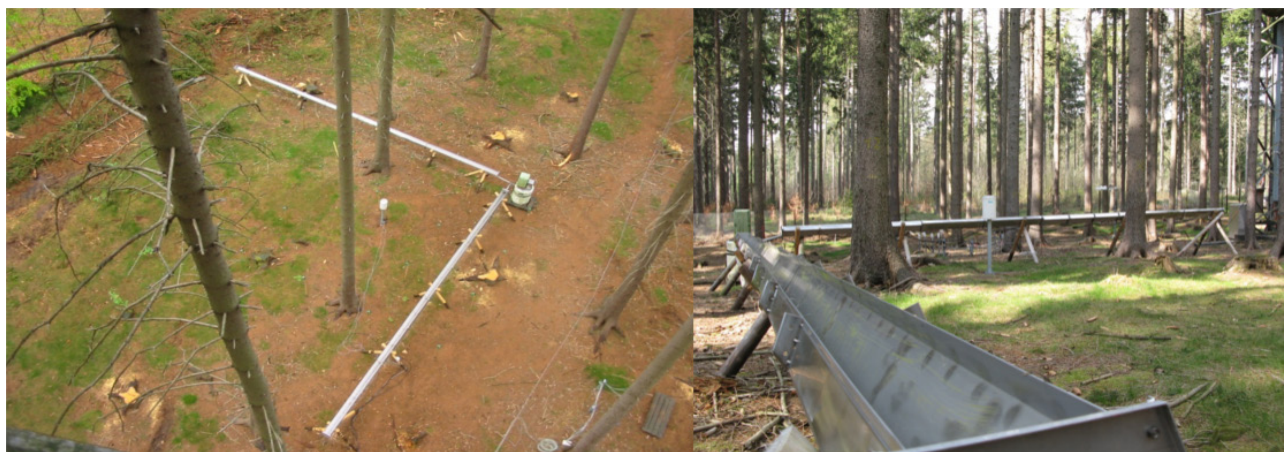
Fig. 1. Examples of throughfall collectors. The centrally collected throughfall collection system and an additional Hellmann precipitation gauge at the Anchor Station Tharandt (spruce site), TU Dresden, Germany.
