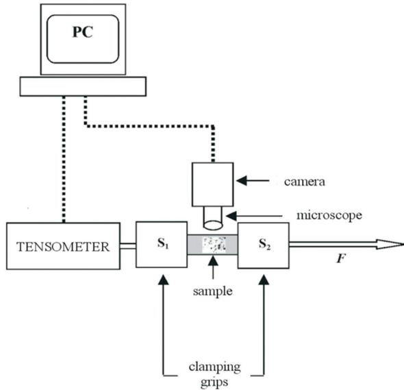
**Fig. 1.** Scheme of the setup used for uniaxial stretching tests. S1 and S2 – clamping grips, F - force.
