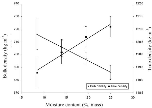
Fig. 3. Effect of moisture content on bulk and true density.
