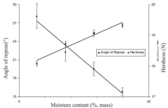
Fig. 4. Effect of moisture content on angle of repose and hardness.
