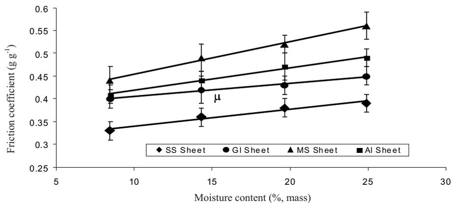
Fig. 5. Effect of moisture content on coefficient of static friction.
