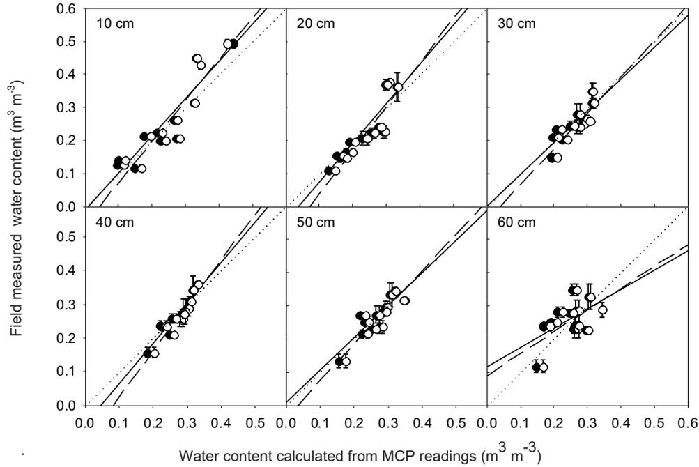
**Fig. 3.** Plot-averaged vs. MCP estimated soil water contents for the mesic Typic Hapludult soil. Solid symbols and hollow symbols show estimates with SENTEK calibration and the laboratory (Starr and Paltineanu, 1997) calibrations respectively. Solid and dash trend lines show the general relationship between plot average and MCP-estimated water contents for SENTEK and the laboratory calibrations. The 1:1 line is the dotted one.
