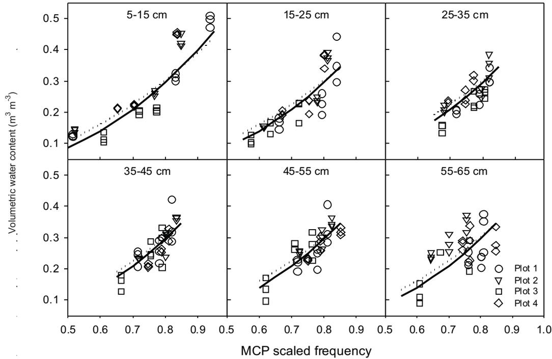
**Fig. 2.** Soil water contents measured in the plots (symbols) and calculated using SENTEK (solid lines) and the laboratory measured (dotted lines) MCP calibrations vs. MCP scaled frequency.
