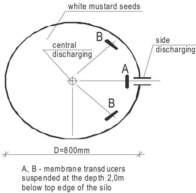
**Fig. 2.** Cross-section of silo bin model showing location of cells and position of side outlet.
