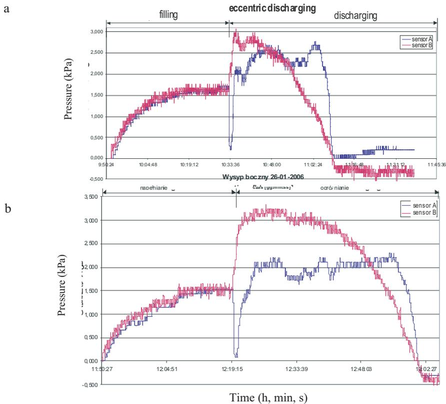
**Fig. 4.** Changes of pressure during filling and discharging phases of the silo model filled with white mustard seeds: a – for cycle 1, b – for cycle 2.
