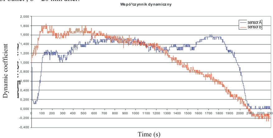
Fig. 6. Changes of dynamic pressure coefficient during discharging process for silo model filled with white mustard seeds.
