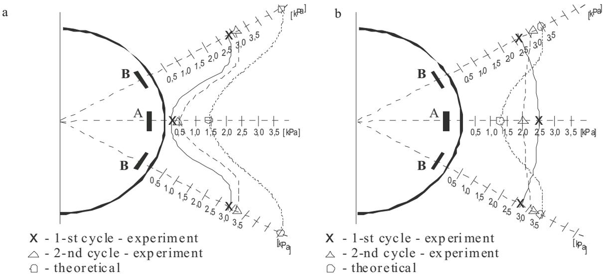
Fig. 5. Comparison of experimental and theoretical lateral pressure values predicted for eccentric discharging of the silo model: a – 1 min after opening of outlet , b – 20 min after.
