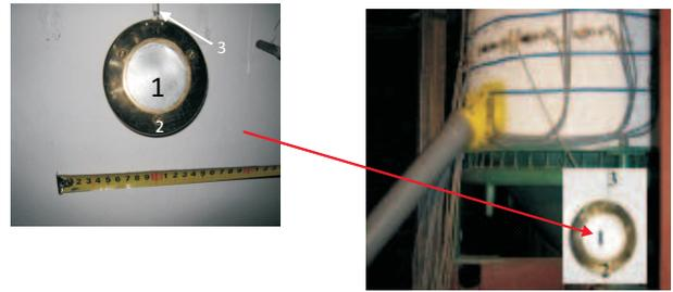
**Fig. 3.** View of silo model with side outlet and embedded cell details: 1 – membrane, 2 – base, 3 – wire.
