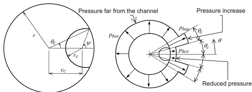
**Fig. 1.** Flow channel during eccentric discharging of silo bin and pressure distribution on silo bin perimeter according to Eurocode 1.
