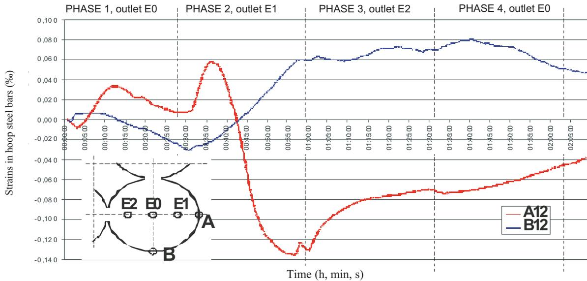
Fig. 7. Strain changes in the real grain silo wall structure due to different modes of discharging.
