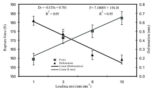
**Fig. 4.** Effects of loading rate on failure force and deformation.
