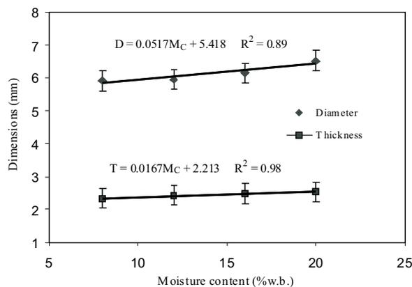
Fig. 1. Dimensions of lentil seed as affected by moisture content.
