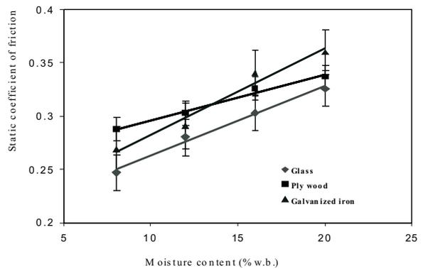
**Fig. 3.** Effect of moisture content on coefficient of static friction of lentil seed against various surfaces.
