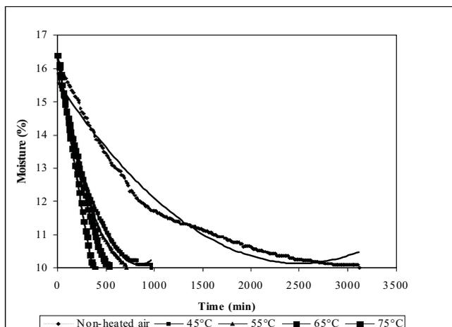
**Fig. 1.** Moisture-time plots for maize dried by five different hot air drying.
