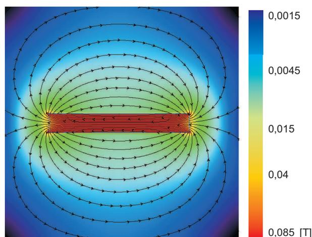
**Fig. 3.** Visualization of the distribution of magnetic field inside of the solenoid, constructed with the help of Vizmag 3.15 (Szecówka, 2008).
