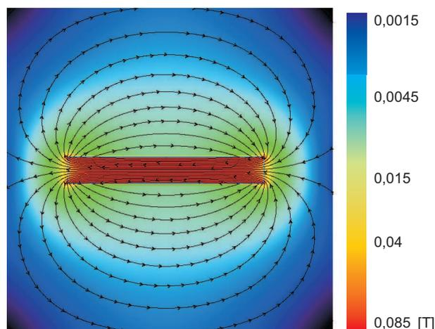
**Fig. 3.** Visualization of the distribution of magnetic field inside of the solenoid, constructed with the help of Vizmag 3.15 (Szecówka, 2008).
