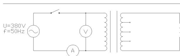
**Fig. 2.** Schematic diagram of electrical system of the solenoid (Szecówka, 2008).
