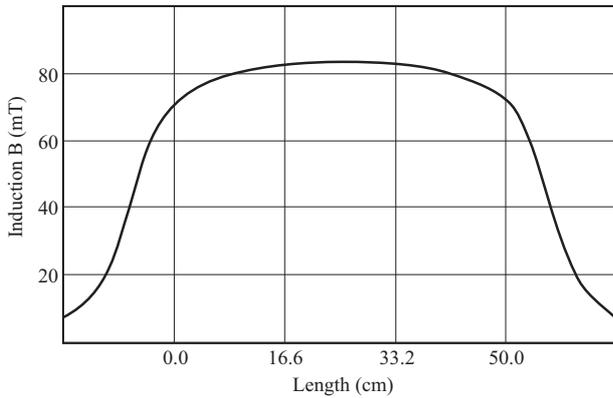
**Fig. 4.** Characteristics of solenoid magnetic induction (Szecówka, 2008).
