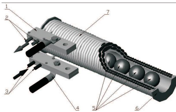
**Fig. 1.** Schematic of the solenoid for magnetic stimulation of seed potatoes: 1 – power supply, 2 – cooling liquid outlet, 3 – coolant inlet, 4 – power cords, 5 – potato tubers; 6 – housing, 7 – winding (Szecówka, 2008).
