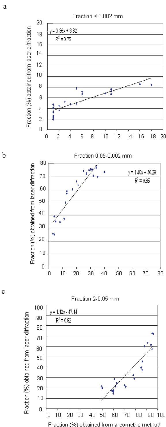
**Fig. 2.** Comparison of for three fraction participations (according to FAO classification) for all soil samples. The results were obtained by LDM and areometric method and calculated according to the Fraunhofer theory.
