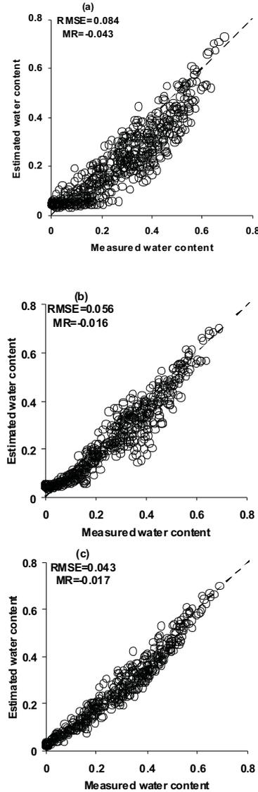
**Fig. 3.** Estimated water content ( $\text{cm}^3 \text{cm}^{-3}$ ) using Rosetta: a – model H3, b – model H4, c – model H5 versus measured one ( $\text{cm}^3 \text{cm}^{-3}$ ) for 59 samples of the GRIZZLY data set.
