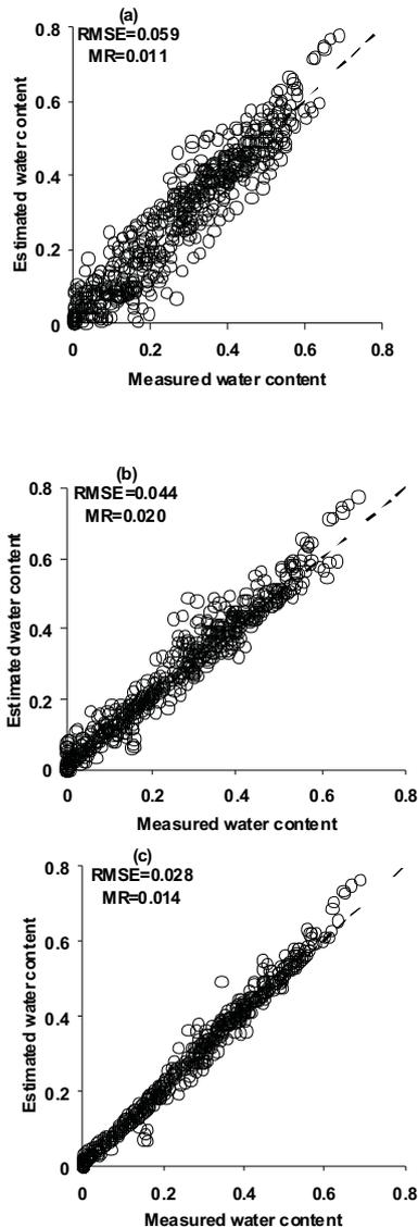
**Fig. 2.** Estimated water content ( $\text{cm}^3 \text{cm}^{-3}$ ) using point PTFs: a – model 1, b – model 2, c – model 3 versus measured one ( $\text{cm}^3 \text{cm}^{-3}$ ) for 59 samples of the GRIZZLY data set.
