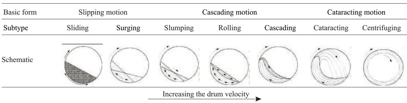
**Fig. 1.** Possible forms of transverse motion of grains in partially-filled, horizontal rotating drums.
