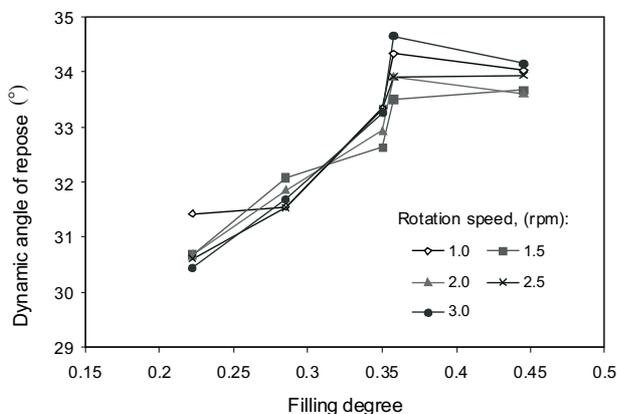
Fig. 10. Effects of filling degree and rotation speed on dynamic AR of wheat grains at 7.5% moisture content.
