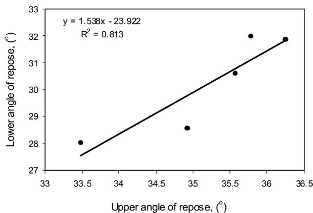
Fig. 9. Correlation between the lower and upper AR of wheat grains measured at 5 different filling degrees.
