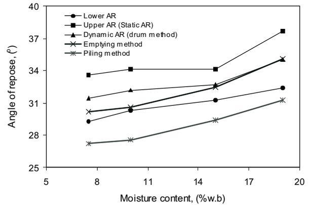
**Fig. 6.** Effect of moisture content on lower, upper, and calculated dynamic AR of wheat grains (filling degree = 0.222, rotation speed = 1 r.p.m.).
