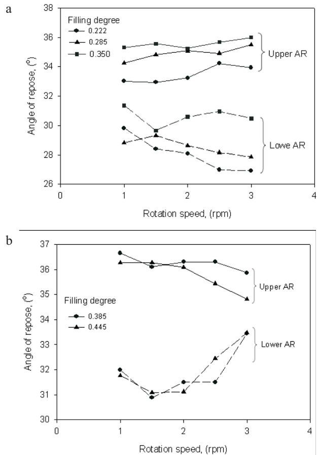
**Fig. 8.** Effect of rotation speed on upper and lower AR of wheat grains at: a – low and b – high filling degrees.
