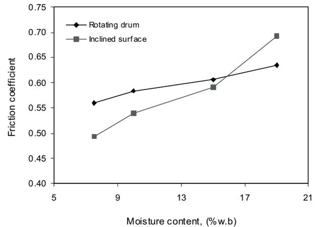
**Fig. 7.** Effect of moisture content and measurement method on friction coefficient of wheat grains (filling degree = 0.222, rotation speed = 1 r.p.m.).
