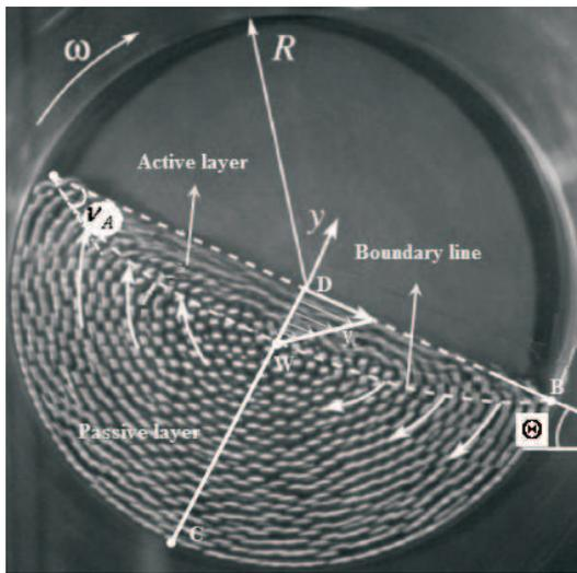
Fig. 3. The parameters of the granular bed in the rolling mode of motion.
