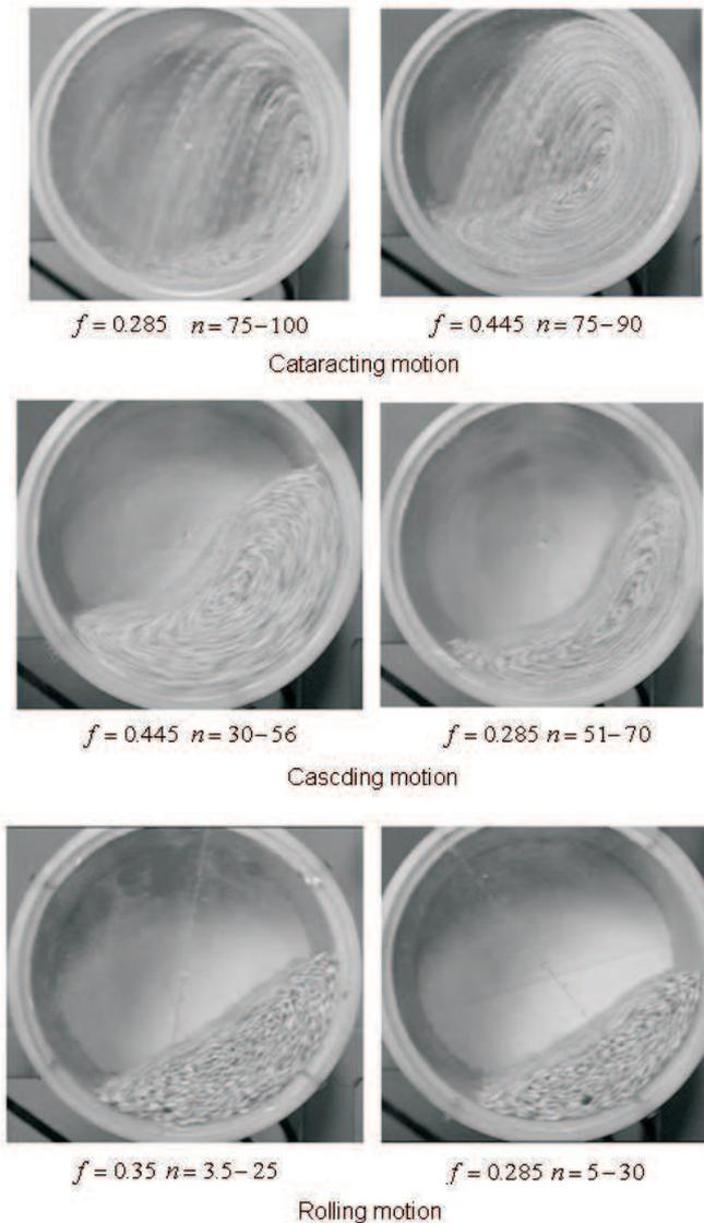
**Fig. 5.** Typical pictures of motion behaviour of wheat grains in the RD at different filling degrees and rotation speed.
