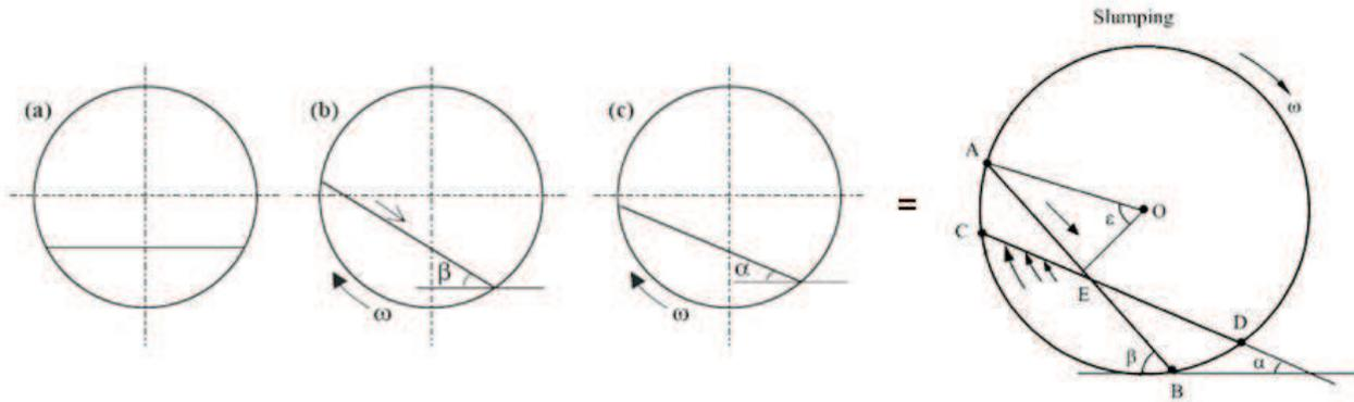
Fig. 2. The slumping mode of motion in the rotating drums.
