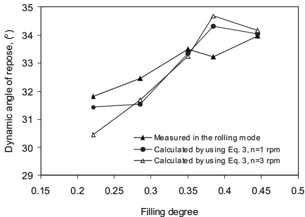
**Fig. 11.** Dynamic AR of wheat grains measured in the rolling mode and its slumping calculated values (Eq. (3)) at two different rotation speeds.
