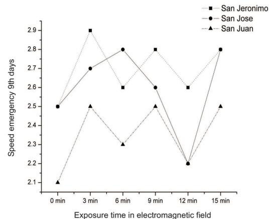
**Fig. 1.** Emergence rate on day 9 of maize hybrid seed with electromagnetic field.
