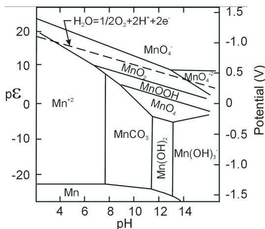
**Fig. 1.** pE-pH diagram for Mn.  $C_T = 2 \cdot 10^{-3} M$ , activity of soluble metals ion species,  $10^{-5} M$ .
