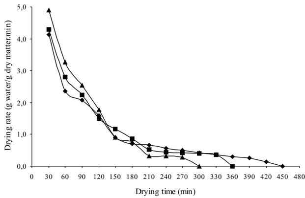
**Fig. 3.** Drying rate ( $\text{g water g}^{-1} \text{ dry matter min}^{-1}$ ) of milky mushrooms dried by fluidized-bed drying method. Legend as in Fig. 1.
