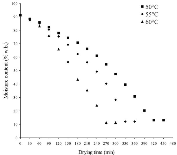
Fig. 1. Variation of moisture content of milky mushroom with drying time during fluidized-bed drying.
