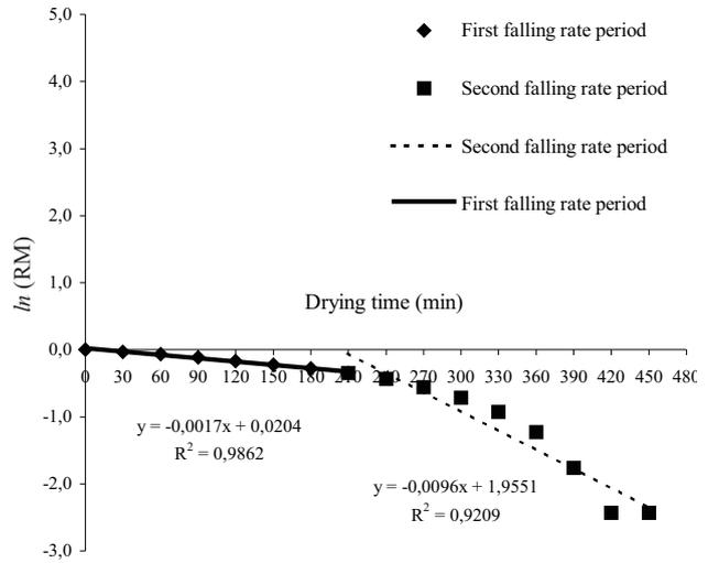
Fig. 4. Relationship between  $\ln(MR)$  and drying time for milky mushroom dried at  $50^\circ\text{C}$ .
