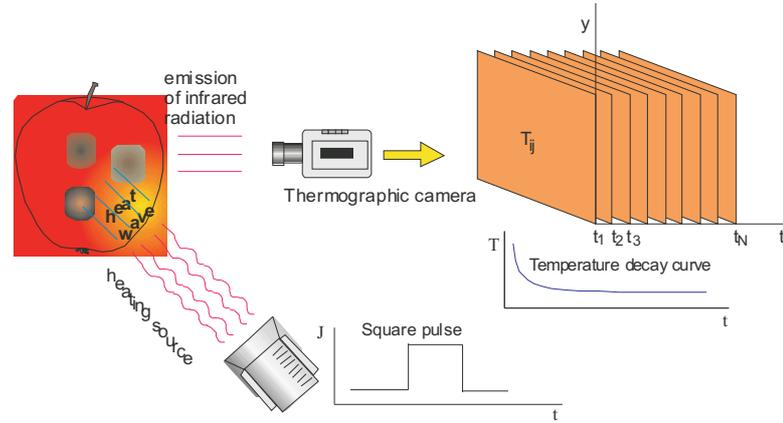
**Fig. 3.** Principle of pulsed-phase thermography (PPT).
