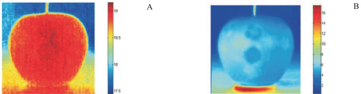
Fig. 6. Thermograms of 'Champion' apple before (A) and after (B) pulse heating.
