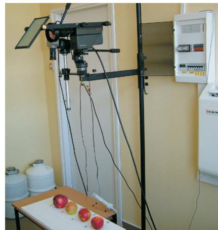
**Fig. 1.** Setup for watercore detection in apples.
