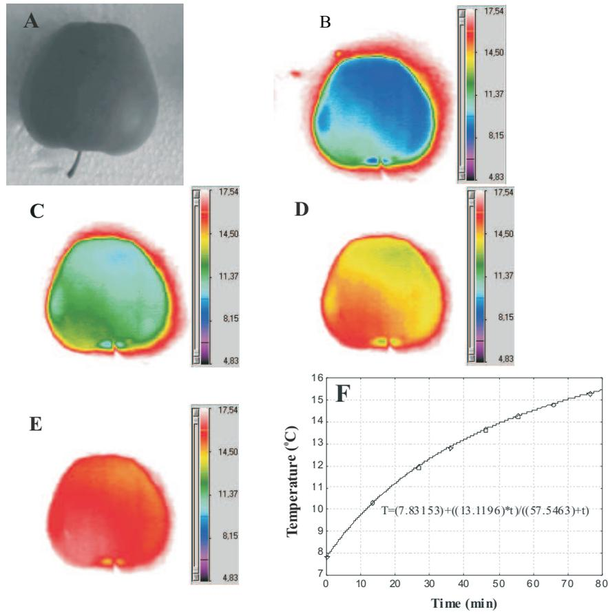
**Fig. 4.** Visible light image of a studied ‘Gloster’ apple (A), a sequence of thermograms during heating process (B-E), measured temperature increase and fitted curve (F).
