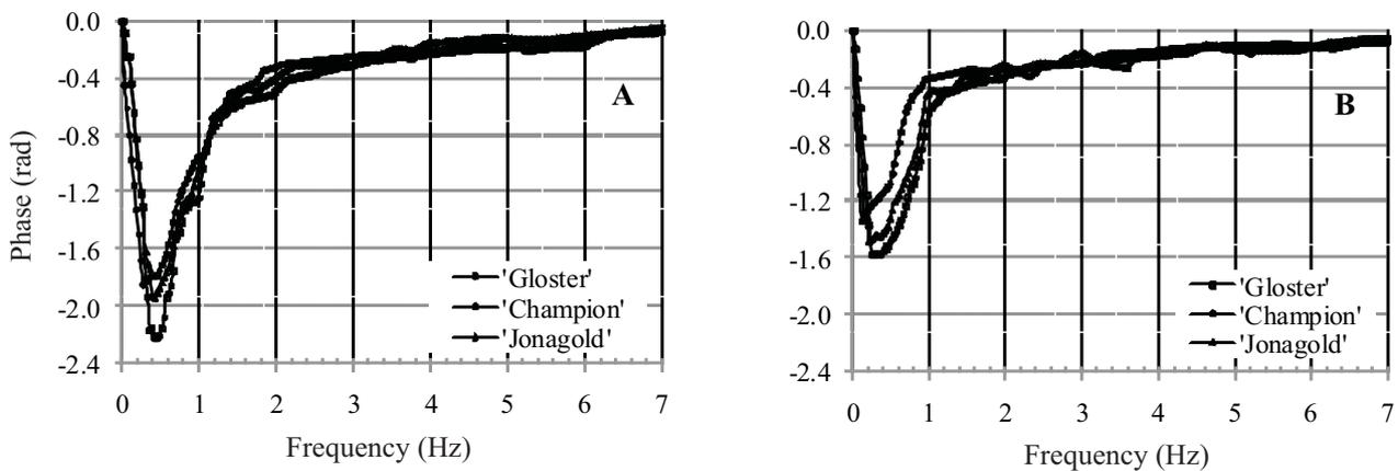
Fig. 7. Change of phase for various frequencies of thermal response in shallower (A) and deeper (B) bruised areas in apples of the three studied varieties.
