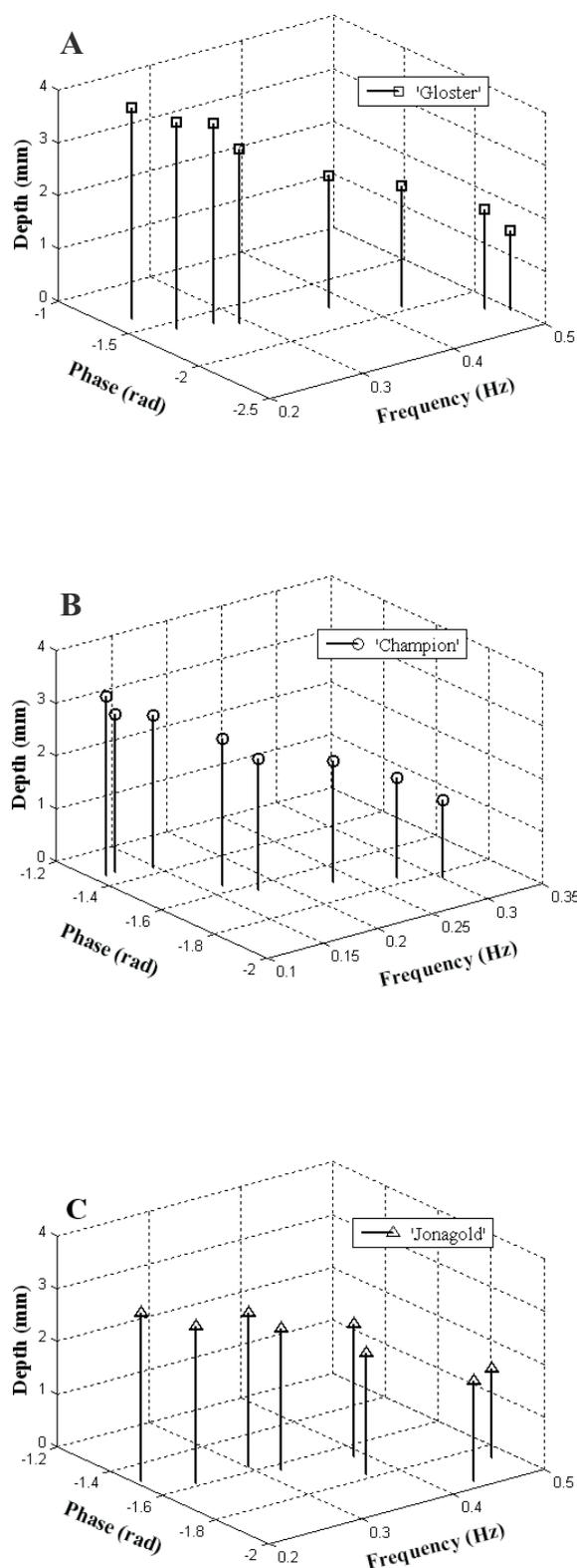
Fig. 8. Relation between bruise depth, minimum peak phase and frequency of thermal response for the studied varieties of apples.
