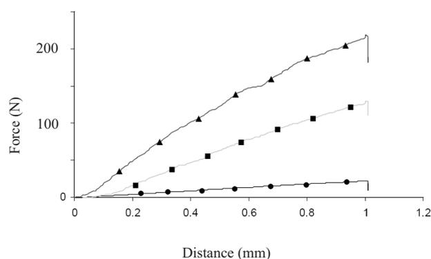
**Fig. 2.** Typical force-deformation plot which resulted from tension loading of a specimen: ▲ upper, ■ middle, and ● lower regions.
