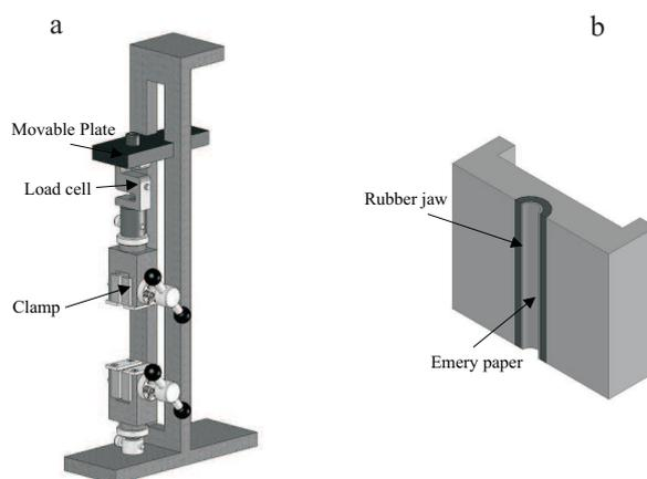
**Fig. 1.** Apparatus for the measurement of tensile strength: a – schematic of apparatus, b – clamp.
