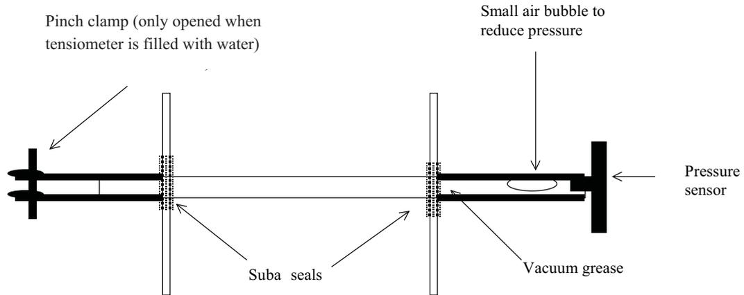
Fig. 4. Home made tensiometers, inserted in the microcosm and filled with de-aired water.
