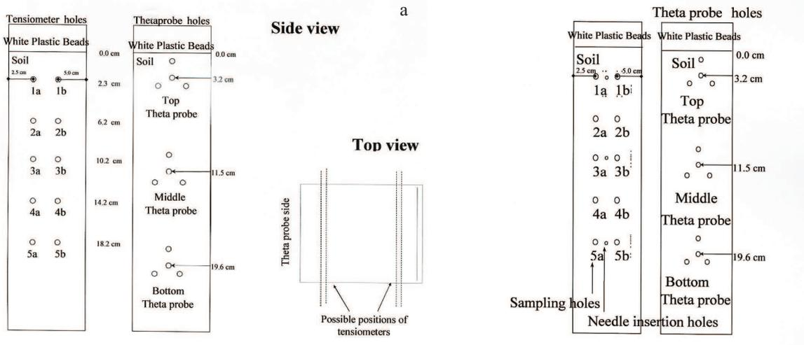
**Fig. 3.** Microcosm, made by a plastic cable conduit and a Perspex plate: 29.8 cm x 7 cm x 6.5 cm: a – used in experiments A, D and E; b – modified microcosm (to allow soil sampling by core) used in experiments B and C.
