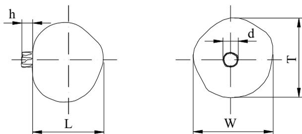
**Fig. 1.** Dimensions of pomegranate, front view (left) and side view (right).
