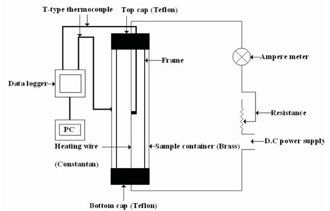
**Fig. 1.** Schematic of the apparatus used for measuring thermal conductivity of dairy cattle manure, PC – personal computer, DC – direct current.
