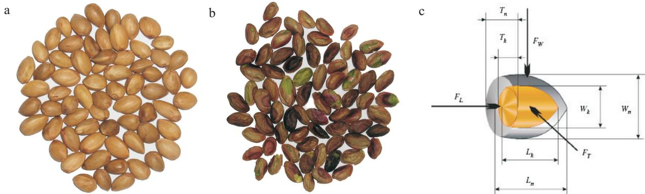
**Fig. 1.** Wild pistachio nuts (a), wild pistachio kernels (b), and (c) characteristic dimensions of wild pistachio nut and kernel and compression directions;  $L_n$ ,  $W_n$ ,  $T_n$  are the length, width and thickness of the nut;  $L_k$ ,  $W_k$ ,  $T_k$  are the equivalent dimensions of the kernel;  $F_L$ ,  $F_W$ ,  $F_T$  are the forces applied in three directions.
