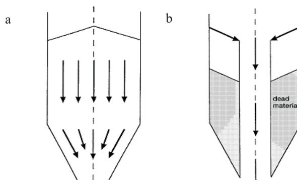
**Fig. 1.** Basic types of granular material flow from a silo: a – mass flow, b – funnel flow (Spencer and Hill, 2001).
