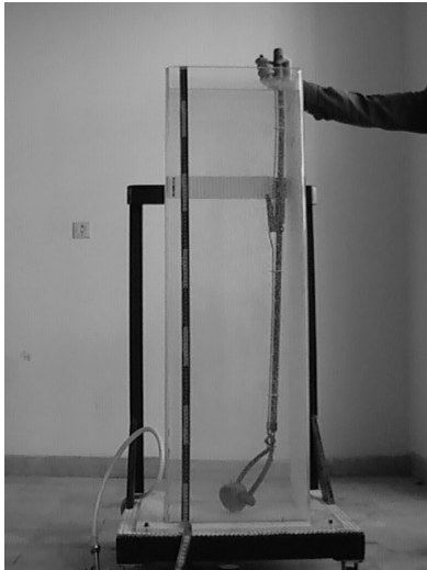
Fig. 2. Water column for determination of hydrodynamic properties. An apple on the bottom of the water column, prepared to be released.
