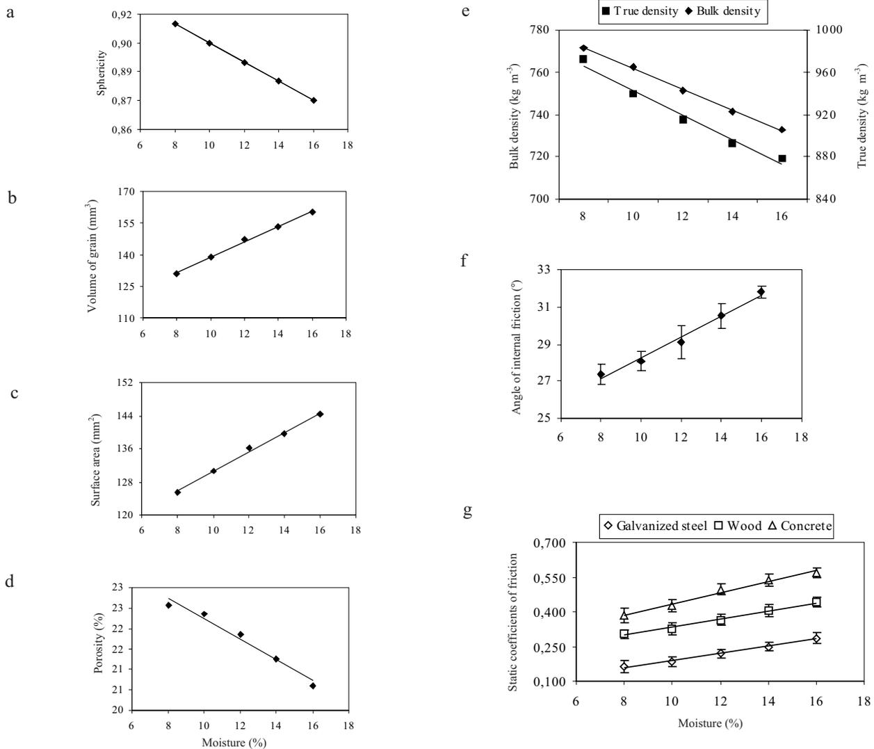
**Fig. 2.** Effect of moisture content on: a – sphericity, b – volume of grain, c – surface area of grain, d – porosity, e – bulk density and true density, f – angle of internal friction, g – static coefficient of friction.
