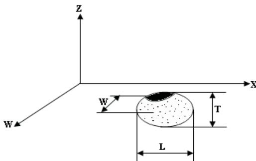
Fig. 1. Characteristic dimensions of soybean.
